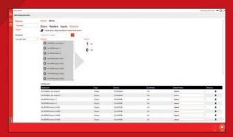
Actions can be configured to operate automatically (e.g. fire alarm), via schedule (e.g. disable alarms during office hours) or via operator instruction (e.g. turn on all the floodlights). All actions are configured in the EntroWatch host and downloaded to the panels for autonomous operation. Peer to peer operation is also supported.
